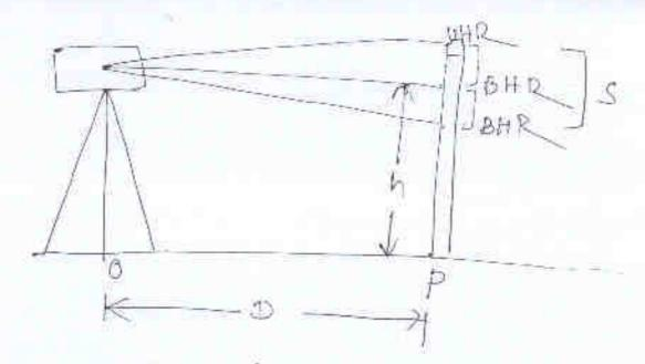
When the line of sight is honizordal the general tacheometry eq? is given by Dt-03.05.21 D=KStC
