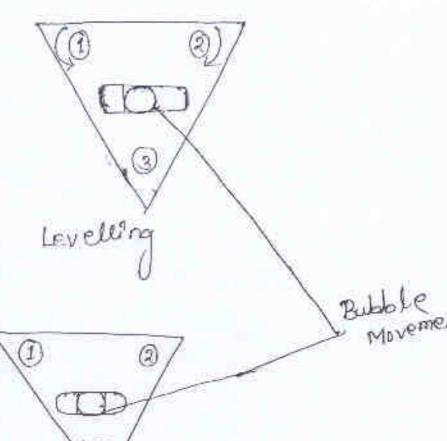
(1) centering is checked by an optical plumment end centre of the enoss hains. if the centre is out nepeal the procedure to make it centre once again. 7 Losen the tripoid base plate screw and use three levelling screw ton time adjustment. 7 For making centering and levelling of the instrument The incurstation of the instrument over the lower plate and movement of the fort screw is done simultaneously. Measurement of angles and distances:-
