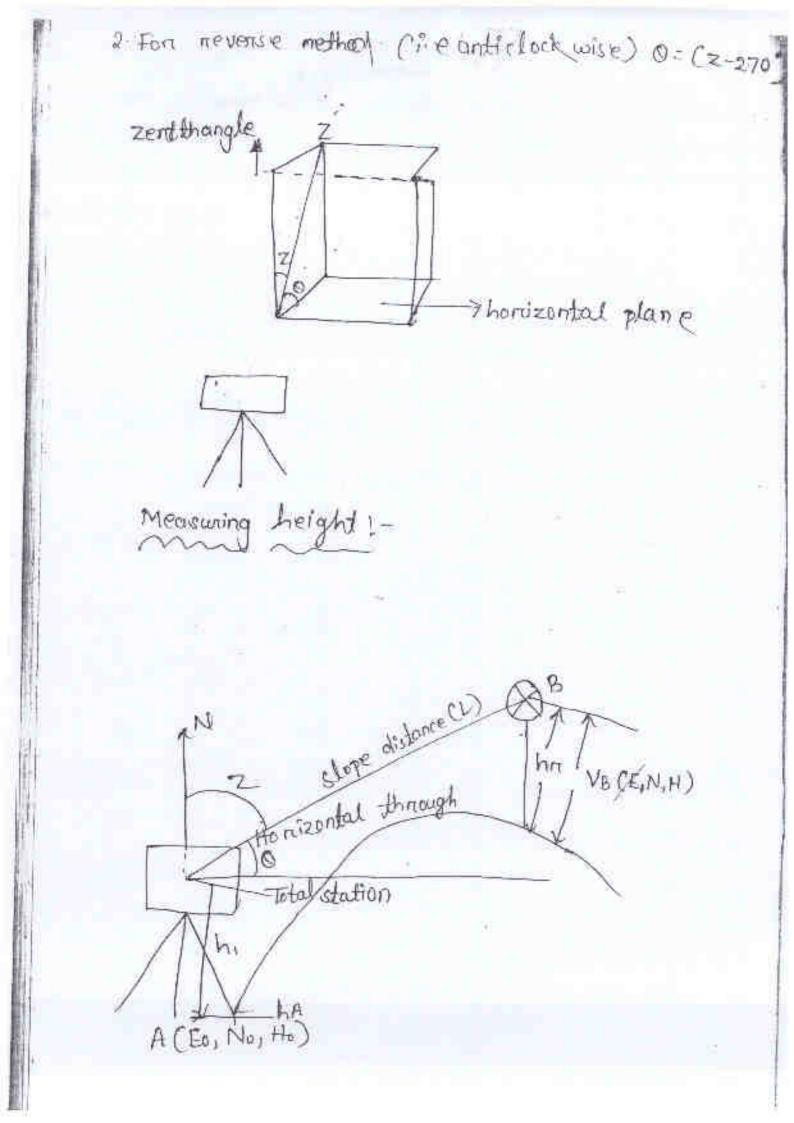
To determine the height by using total station zand o vertical angle bet " A and B' be the zenith and can be calculated.
