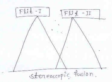
7 In wonial photography when photographs overlap on the some ground area is photograoverlap on the some ground area is photograph fram two separate position forms a stone pain used for three dimensional viewing thus obtaining pain were fore three dime in the obtaining pain were fore three dime prional veiwing . of storeoscopic photographs on images can be verwed to determine porrall and 3D veiwing.
