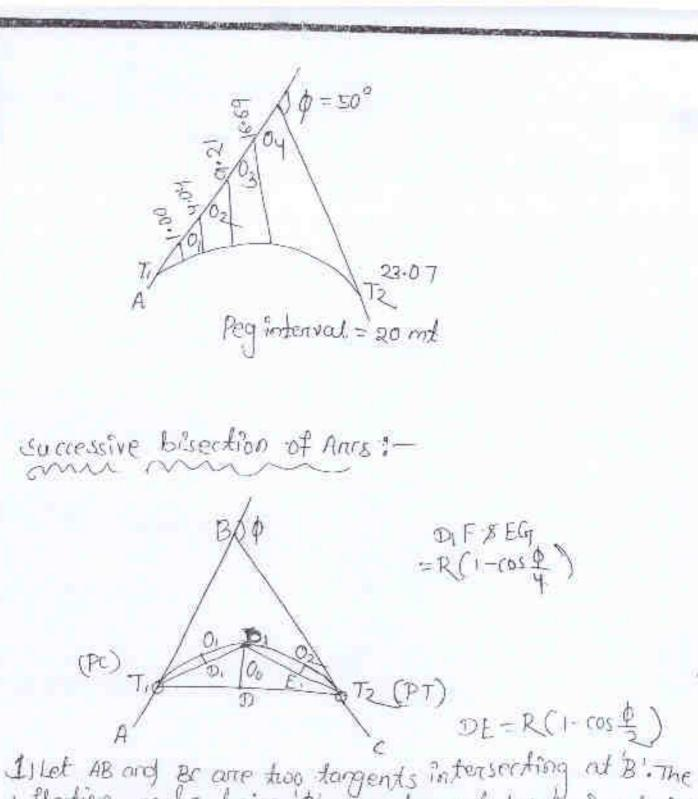
Is let AB and BC are two targents intersecting at B'. The deflection angle being Q'. The targent length is calculated and forgent points T, and Tz are marked on the around with pegs.
